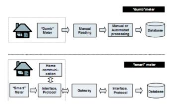
Figure 1: Different between convectional metering and smart metering. [6]
