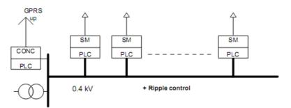
**Figure 3:** Smart meters with PLC communication. [7]
